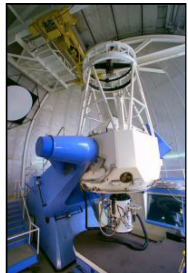
The actual 2.1-meter telescope. The white spot on the dome (to the left) is used to calibrate the spectrograph.
